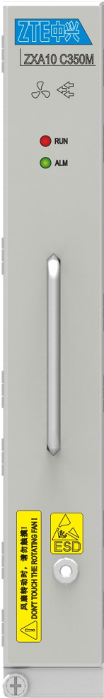
Figure 3-54 Panel of the ZXA10 C350 Fan Box
